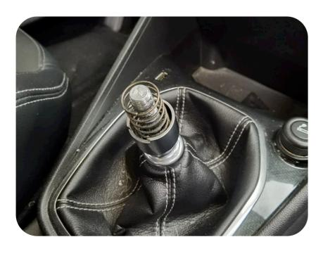
Once the knob is unscrewed, clean well the thread and the spring from the grease. A piece of paper is enough.
